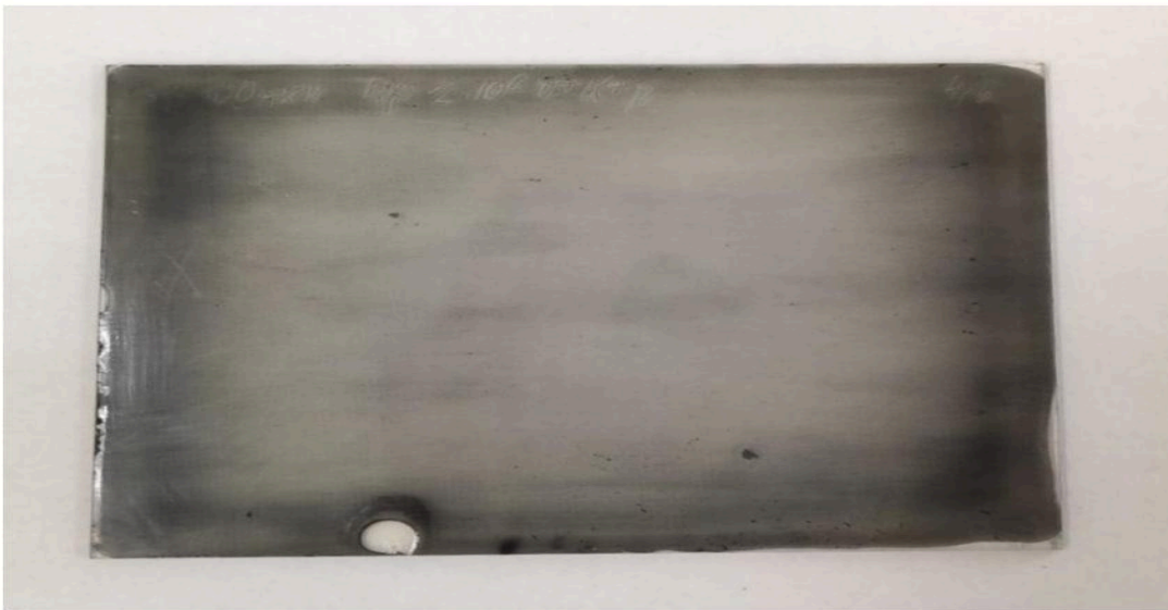
Fig. 1. NTE plate after chemical development. The typical size of NTE plate is 9 \times 12 \text{ cm}^2 with around 100 \mu\text{m} thickness of sensitive emulsion layer.
