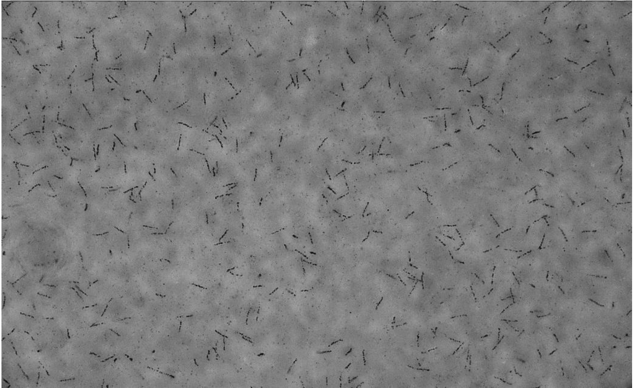
Figure 5: High resolution photograph of traces in emulsion taken with Olympus BX63 microscope
