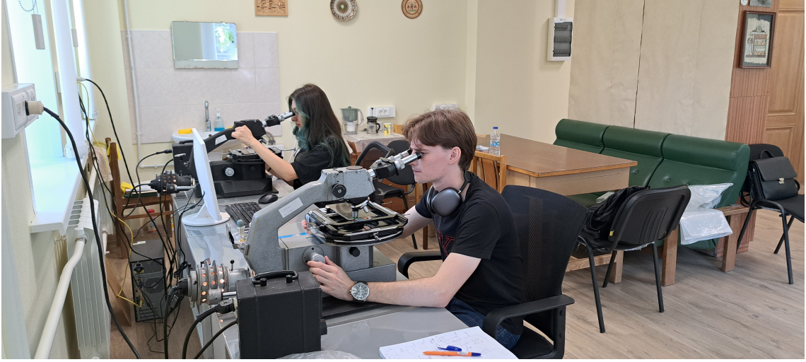
Figure 4: Beam profile measurement using the MBI-9 microscope
