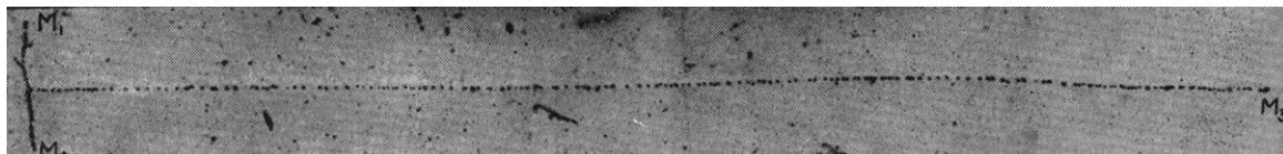
Fig. 1. TRIPARTITION OF URANIUM NUCLEUS WITH LIGHT THIRD FRAGMENT (ITS RANGE IN STANDARD AIR = 44 CM.). THE TWO BRANCHES ON M_1 TRACK ARE DUE TO NUCLEAR COLLISIONS OF M_1 WITH KNOWN NUCLEI CONTAINED IN PHOTOGRAPHIC EMULSION m_1 = 110 , m_2 = 120 , m_3 = 6 \pm 1 . Total kinetic energy \sim 179 MeV.
