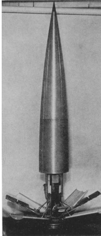
Fig. 15. Aerobee nosecone designed for the collection of meteoritic dust. Some of the pockets can be fitted with small emulsion blocks.
