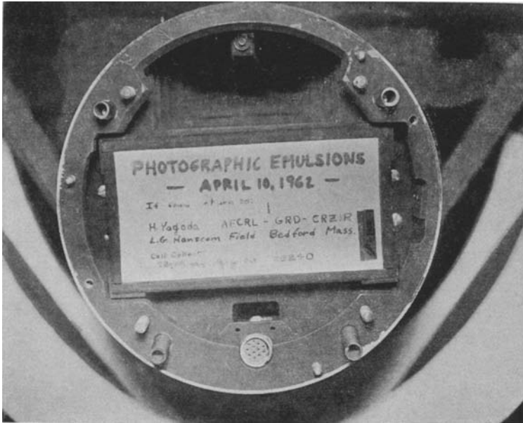
Fig. 13. Orientation of emulsion block on Aerobee rocket designed to study auroral spectra.
