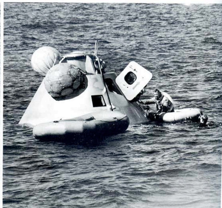
"Stable two," an engineering euphemism for upside-down, was one of the ways that the command module could float, and this was the way that Apollo 7 splashed down. The astronauts hung from their restraining belts for a few minutes until three righting bags were inflated to flip the spacecraft. The photo sequence above and at right, not the actual Apollo 7 landing, shows a training session, one of many constantly held to drill recovery teams and astronauts. Not used in this exercise was the flotation collar, normally fixed around the command module, that provided insurance against swamping from water taken aboard through the open hatch.
