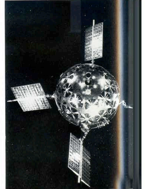
An unsuccessful effort to orbit the Moon was made with the Atlas-Able launch vehicle (above) and the Pioneer P-31 spacecraft (below). The launch vehicle was capable of injecting 380 lb into a translunar trajectory. The 39-in. spacecraft carried two 18.5-lb-thrust liquid-propellant engines for flight-path corrections and injection into lunar orbit.
