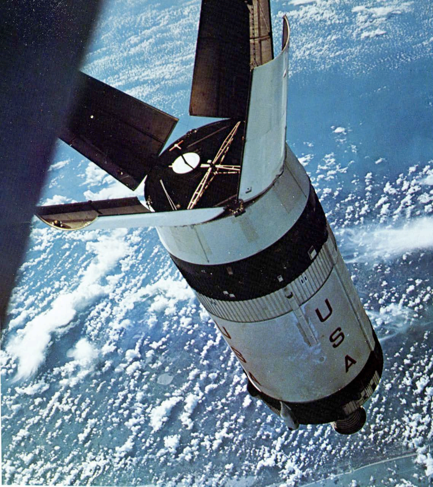
Lifeless and slowly tumbling , the S-IB stage that put Apollo 7 in orbit gave Astronauts Schirra, Eisele, and Cunningham man's first ride atop a load of liquid hydrogen. Now the spent 59-foot stage served as a passive target for practice in rendezvous, with one run starting from a distance of 80 miles.
