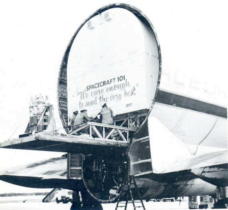
Snug-fitting cocoon housing the Apollo 7 service module is carefully extracted by workmen from the Super Guppy , the specially built cargo transport plane. The SM will be mated with its CM and then fully tested to confirm compatibility.
