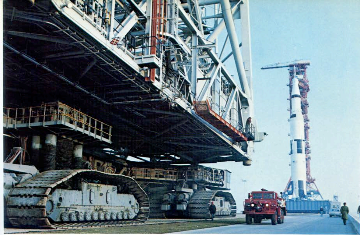
The Mobile Service Structure coming down from the launch pad. About 11 hours before launch, a crawler carries the MSS back from the pad to its parking area. Although the crawler is descending a 5-degree slope, the hydraulic cylinders, shown here fully extended, keep its platform level.
