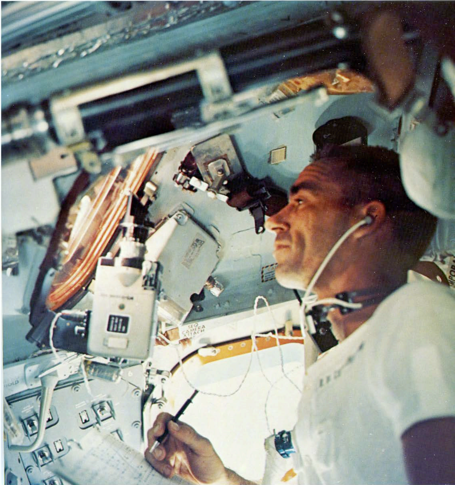
Like new Magellans , astronauts learned to navigate in space. Here Walt Cunningham makes his observations through a spacecraft window. The tools of a space navigator included a sextant to sight on the stars, a gyroscopically stabilized platform to hold a constant reference in space, and a computer to link the data and make the most complex and precise calculations.
