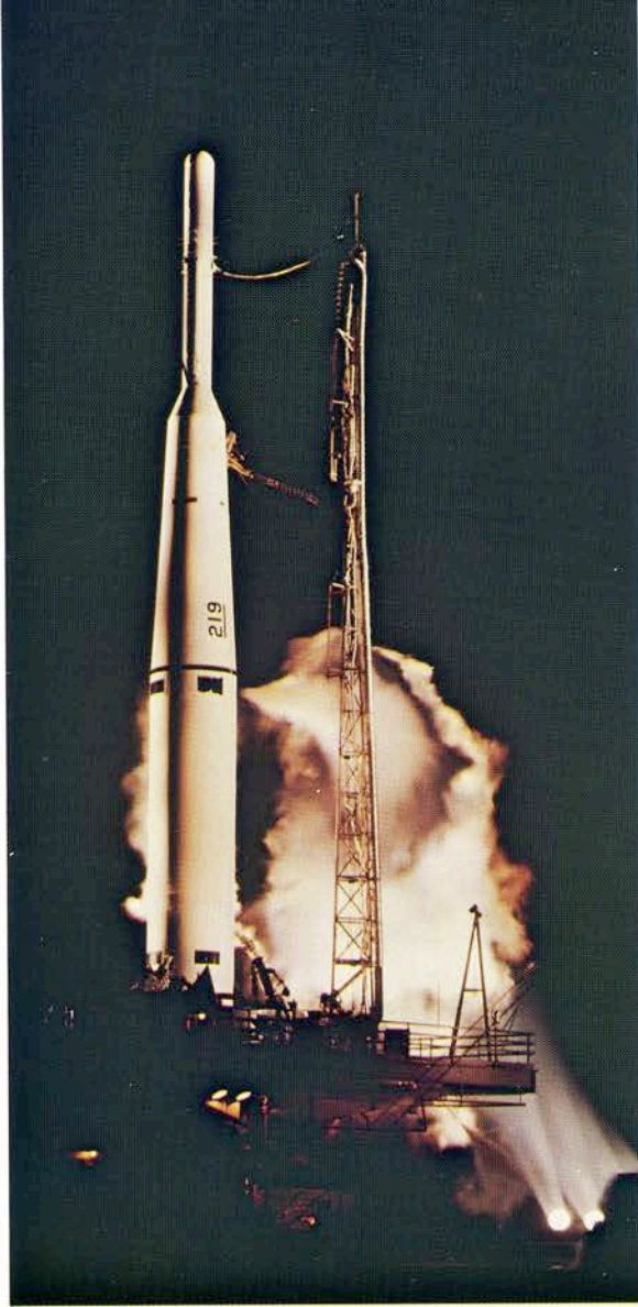
The Thor-Able, with more advanced upper stages, propelled the 94.4-lb Pioneer V spacecraft to escape velocity on March 11, 1960. The instrumentation of this payload (below) measured the Earth's outer magnetosphere, detected an interplanetary magnetic field, helped explain the effect of solar flares on cosmic rays, and first detected the plasma clouds emitted by the Sun during solar storms. But it told nothing new about the Moon.
