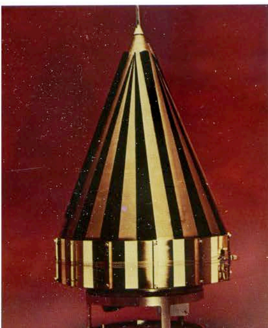
A Juno II launch vehicle was made up of an Army Ballistic Missile Agency's modified Jupiter first stage with a spin-stabilized solid-rocket upper stage developed by the Jet Propulsion Laboratory. JPL also developed the 13.4-lb Pioneer IV payload shown below. Launched March 3, 1959, it helped detect and measure the second of the Earth's great radiation belts.
