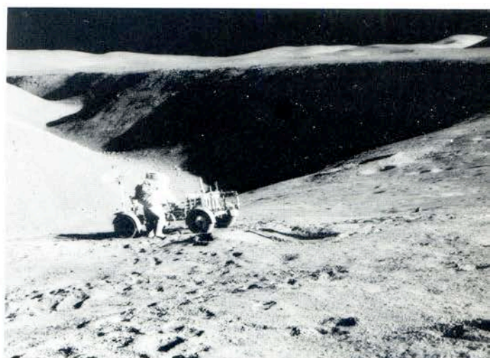
Parked by Hadley Rille in the first of the traverses shown at left above, the Apollo 15 Rover had already displayed its workhorse willingness. It weighed 462 pounds (but only 77 on the Moon), and could carry two suited astronauts, their gear and cameras, and several hundred pounds of bagged samples.
