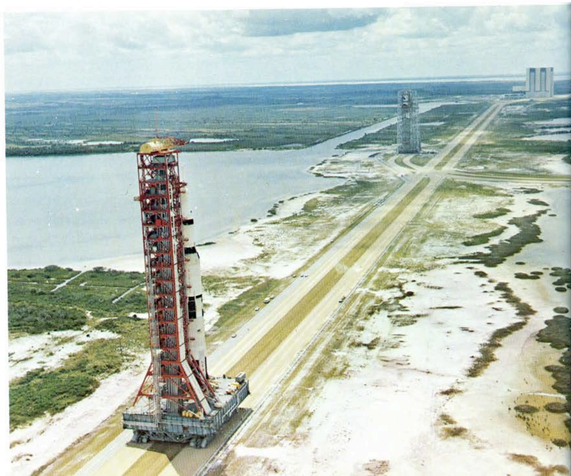
The first Saturn V space vehicle and its Mobile Launcher on their way out to Launch Pad A atop a transporter. The pad is 3½ miles east of the VAB. The Mobile Service Structure is parked at the loop where the crawlerway to Pad B diverges to the north (right). The barge canal to the VAB runs parallel to the main crawlerway.
