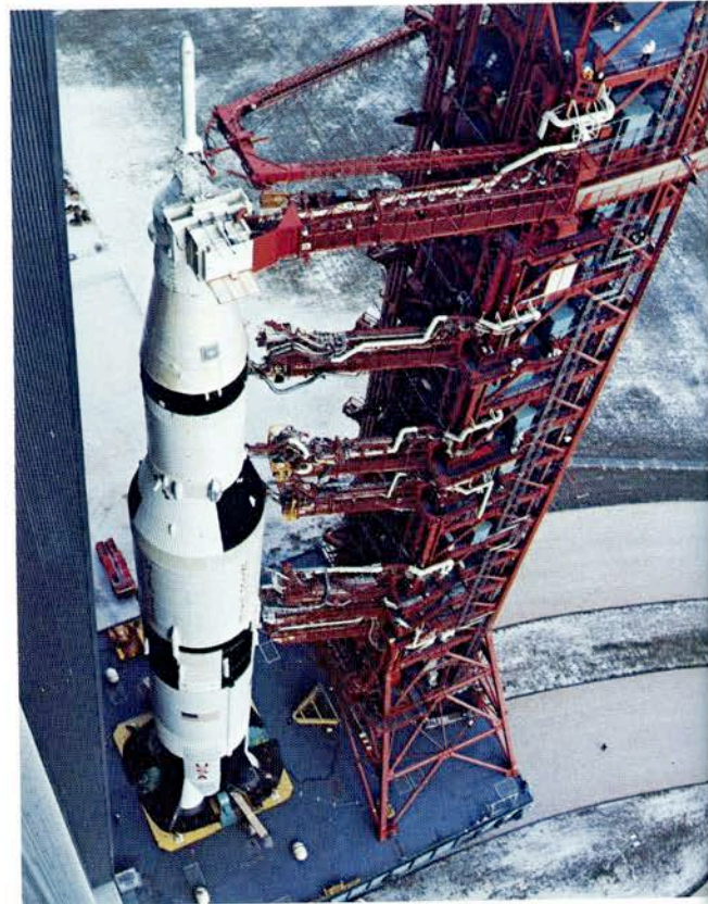
Looking down at the space vehicle as it leaves the VAB on the base platform of the Mobile Launcher. The nine swing arms that run from the launcher's tower to the vehicle's various levels are in extended position.
