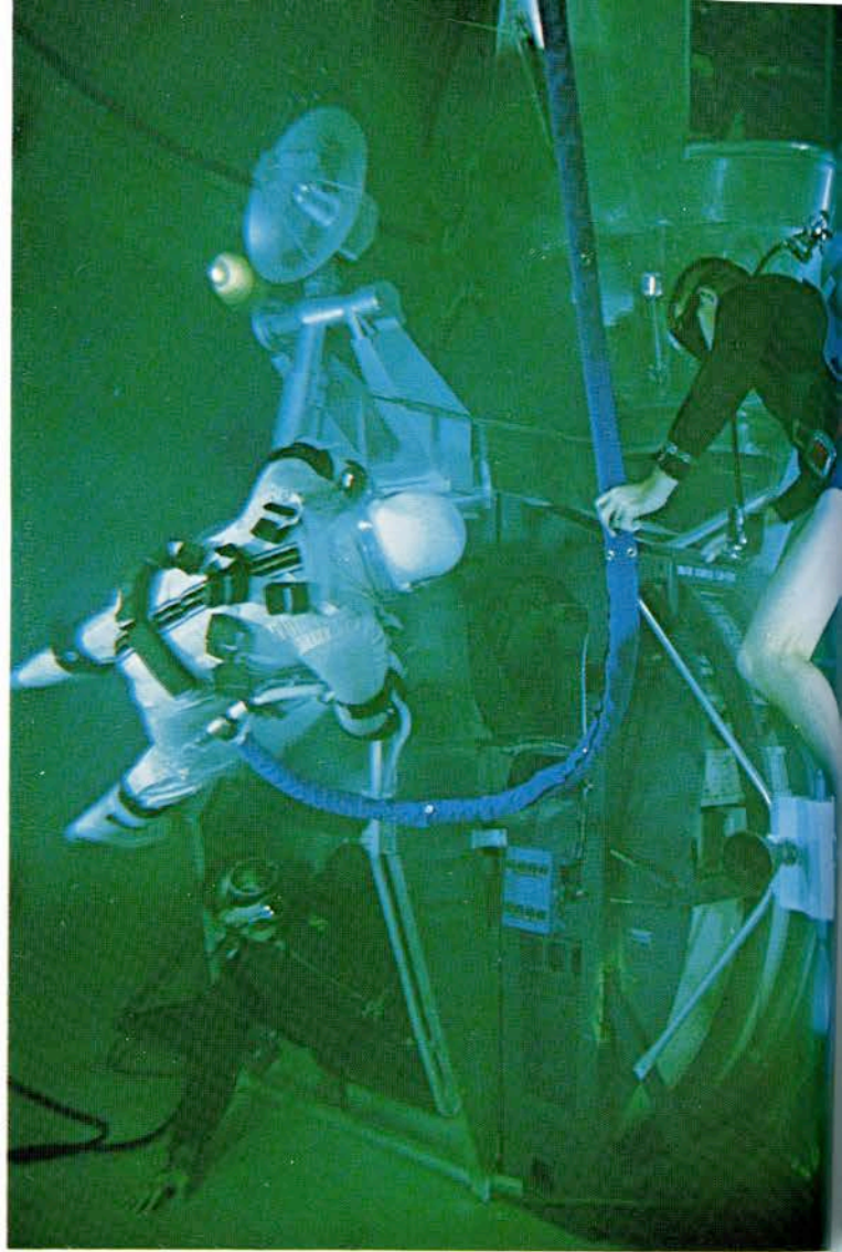
A parabolic flight path in a jet transport could create up to 30 seconds of zero gravity, enough to practice exit through a spacecraft hatch (above). Two earth-bound simulations of reduced or zero gravity are shown at right and below. Wearing pressure suits carefully weighted to neutral buoyancy, astronauts in a big water tank learn the techniques needed to work effectively in space. Below, ingenious slings are supported by wires running to a trolley high above. The angled panels on which the man walks or runs are offset just enough from directly under the trolley to simulate the sixth of Earth gravity that prevails on the Moon.
