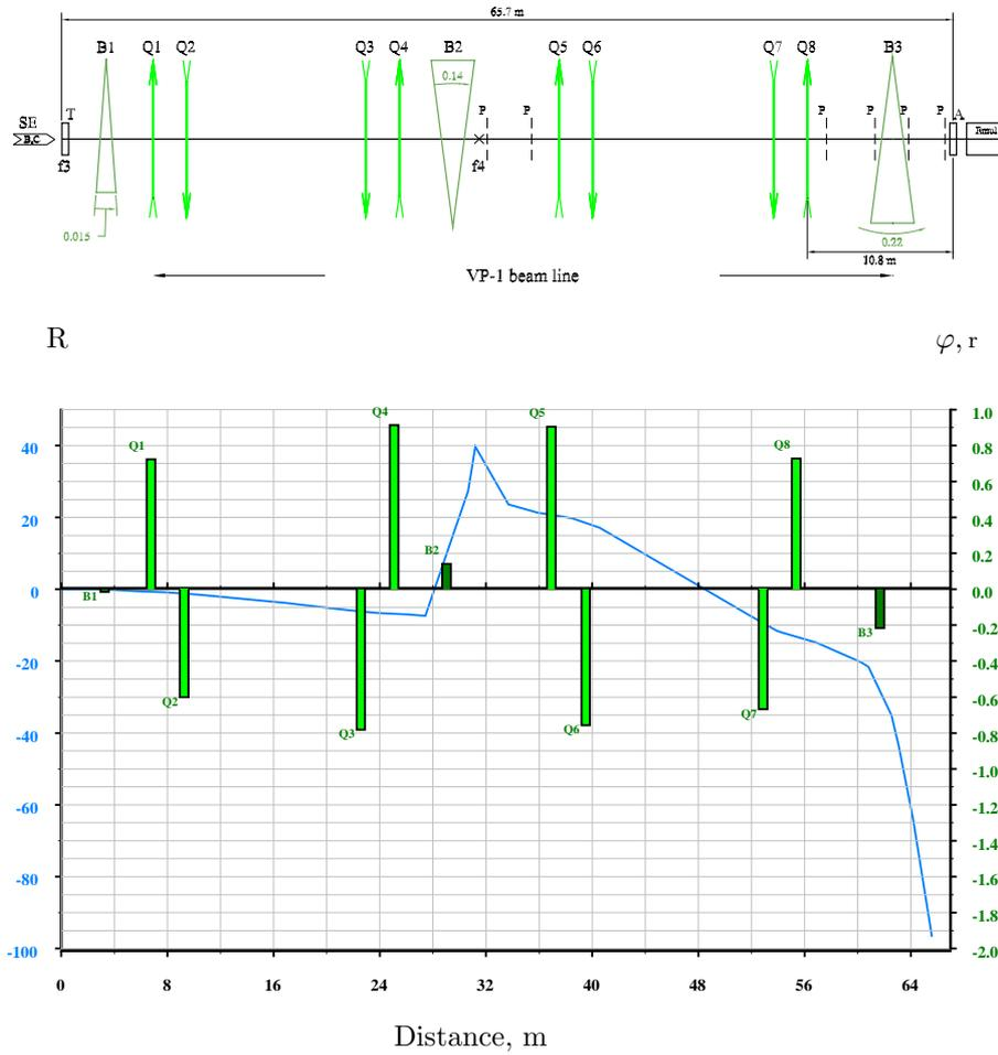
Fig. 1. Above: scheme of secondary nuclear fragment beam forming. Q1...Q8 - quadrupole lenses, B1...B3 - dipole magnets, T - target, A - beam analyzer, P - profilemeters, SE - primary slowly extracted beam. Below: a beam line regime. The vertical bars - states of the magnetic elements,  $\varphi: (eB/pc)l_{eff}$  (bend angle) and  $\sqrt{eG/pc}l_{eff}$  for magnets and lenses correspondingly. The curve - realized resolution function  $R(z)$  (see in the text).
