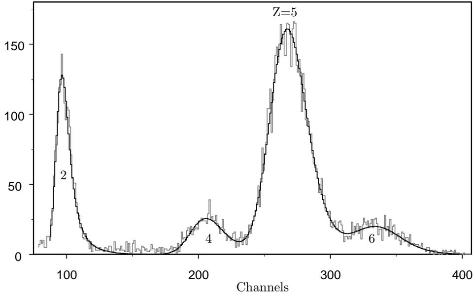
Fig. 2. Energy deposition spectrum in a 5 mm scintillator measured in a secondary beam enriched with  $^8B$  nuclei at 2 A GeV/c momentum. Fraction of the nuclei ( $Z=5$ )  $\simeq$  62%.
