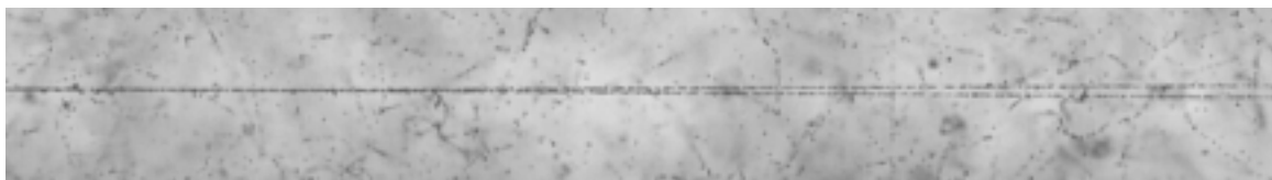
Fig. 1. Fragmentation of the relativistic {}^9\text{Be} nucleus into two He fragments in the emulsion (white star). The photograph is obtained at the PAVIKOM measuring facility at the Lebedev Physical Institute.
