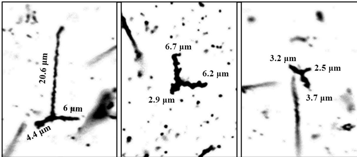
**Figure 1.** Examples of observed events of ternary fission; track lengths are specified. Left photo: long-range  $\alpha$ -particle (long arrow), fragment (middle arrow). Mid and right photo: three fragment tracks.
