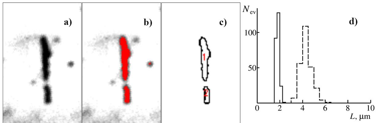
**Figure 3.** Example of disintegration of boron nucleus by thermal neutron to the Li and He  $n_{th}$  (a) and steps of image recognition via the ImageJ program (a-c). Distribution of mean range of Li (solid line) and He (dotted line) (d).
