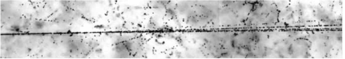
Fig. 1. Event of the 1.2 A GeV  $^{14}\text{N}$  fragmentation in emulsion without target-nucleus excitation or meson production. The interaction vertex and a fragment jet in a narrow angle cone are seen on the photograph. Following the direction of the fragment jet (bottom part) it is possible to make out 3 fragments with  $Z = 2$  and 1 fragment with  $Z = 1$ .
