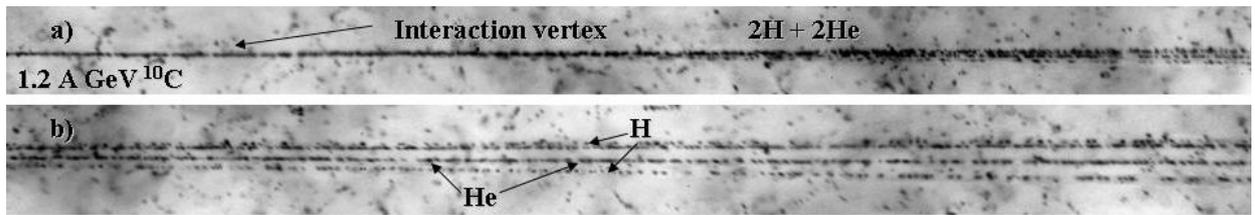
**Figure 1.** Macrophoto of the coherent dissociation event of 1.2 A GeV  $^{10}\text{C}$  nucleus into pairs of He and H nuclei; a) primary track, approximate position of interaction vertex and appearance of fragment tracks and b) tracks of fragments are resolved; opening angles between tracks are  $\Theta_{2\text{He}} = 5.9$  mrad,  $\Theta_{\text{HeH}} = 8.6, 16.6, 3.0, 17.6$  mrad,  $\Theta_{2p} = 20.1$  mrad. Both  $2\text{HeH}$  triples in the event correspond to  $^9\text{B}$  decays.
