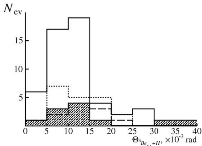
**Figure 6.** Distributions over the opening angle  $\Theta(^8\text{Be}_{g.s.} + \text{H})$  in “white” stars  $^{10}\text{C} \rightarrow ^8\text{Be}_{g.s.} + 2\text{H}$  (solid histogram),  $^{11}\text{C} \rightarrow ^8\text{Be}_{g.s.} + 2\text{H}$  (dashed histogram),  $^{10}\text{B} \rightarrow ^8\text{Be}_{g.s.} + \text{H}$  (hatched histogram) all found stars  $^{11}\text{C} \rightarrow ^8\text{Be}_{g.s.} + 2\text{H}$  (dotted histogram).
