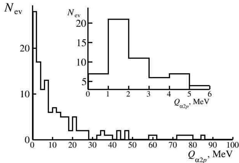
**Figure 4.** Distributions over energy  $Q_{\alpha 2p}$  in measured “white” stars  $^7\text{Be} \rightarrow \text{He} + 2\text{H}$ ; insertion; the enlarged  $Q_{\alpha 2p}$  distribution in the  $^6\text{Be}$  region.
