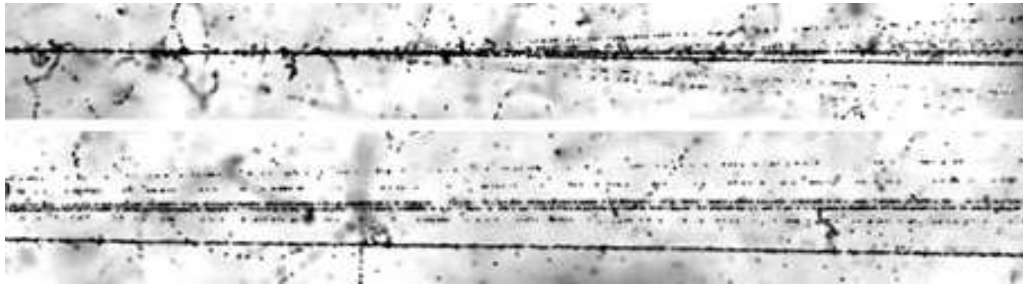
Fig. 12. Event of dissociation of a 4.5A \text{ GeV}/c ^{24}\text{Mg} nucleus in peripheral interaction into charged topology 1+1+2+2+1+5 (from top to bottom). Upper photo: interaction vertex with production of a narrow fragment jet accompanied with a relativistic meson like track. Lower photo: shifting from vertex allows one to resolve six relativistic fragments.
