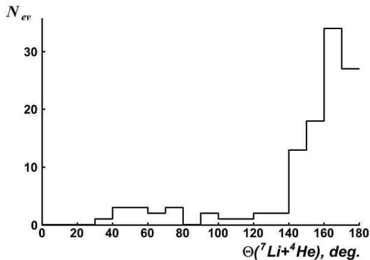
FIG. 1: Distribution over the opening angle  $\Theta(^7\text{Li}+^4\text{He})$  for pairs of  $^7\text{Li}$  and  $^4\text{He}$  nuclei produced by thermal neutrons in 112 events  $n_{th} + ^{10}\text{B} \rightarrow ^7\text{Li} + (\gamma) + ^4\text{He}$ .
