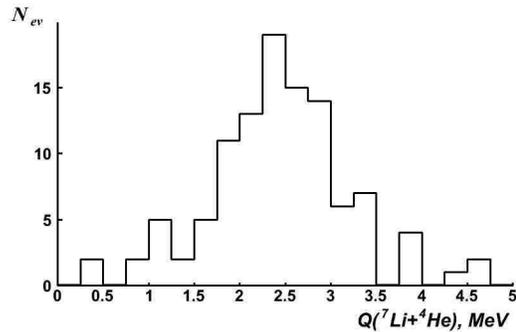
FIG. 2: Distribution over the energy  $Q(^7\text{Li} + ^4\text{He})$  for pairs of  $^7\text{Li}$  and  $^4\text{He}$  nuclei produced by thermal neutrons in 112 events  $n_{th} + ^{10}\text{B} \rightarrow ^7\text{Li} + (\gamma) + ^4\text{He}$ .
