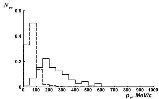
FIG. 7: Distribution over the total transverse momentum  $P_T$  of 72 triples of  $\alpha$ -particles in NTE exposed to  $\mu$ -mesons (solid histogram) and 400 triples of  $\alpha$ -particles from reaction  $n(14.1) + ^{12}\text{C} \rightarrow 3\alpha + n$  [3] (dashed histogram); normalization of the histogram to the number of events.
