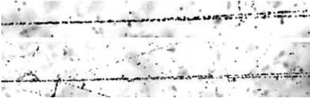
FIG. 9: Examples of peripheral dissociation of 1.23 A GeV  ${}^7\text{Be}$  nuclei into pairs of He nuclei. Upper photo: dissociation without target nucleus excitation and produced charged mesons. Lower photo: dissociation accompanied by a target fragment and a meson like pair.
