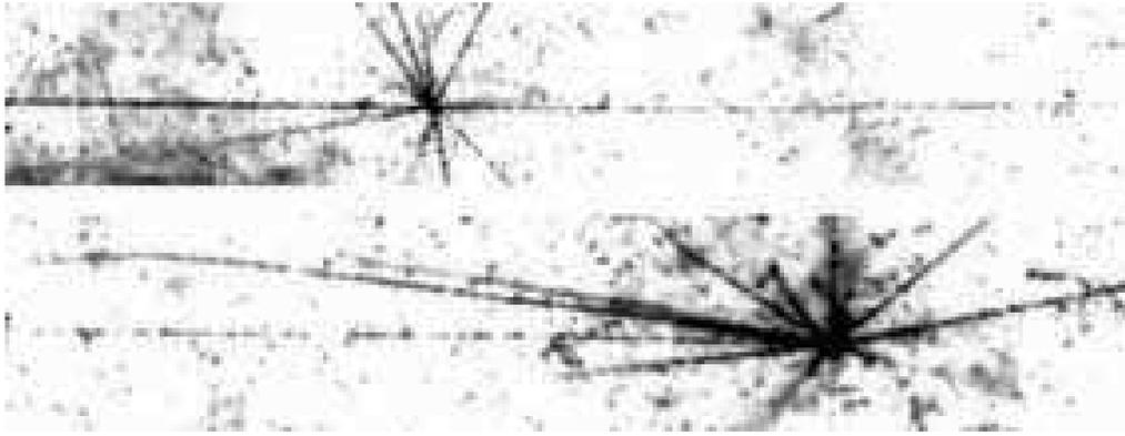
FIG. 8: Event of a 2.67 A GeV  ${}^6\text{He}$  nucleus interaction with fragmentation into a relativistic  $\alpha$  particle. The  $\alpha$  particle track is followed until a violent inelastic interaction.
