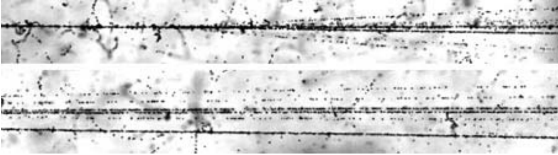
Figure 12: Event of dissociation of a 4.5A GeV/c ^{24}\text{Mg} nucleus in peripheral interaction into charged topology 1+1+2+2+1+5 (from top to bottom). Upper photo: interaction vertex with production of a narrow fragment jet accompanied with a relativistic meson like track. Lower photo: shifting from vertex allows one to resolve six relativistic fragments.
