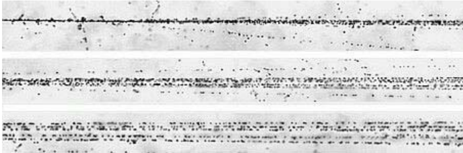
Figure 1. 4.5-A GeV/c ^{24}\text{Mg} nucleus dissociation into five double and two single charged fragments in sequential evaluation (top to bottom).
