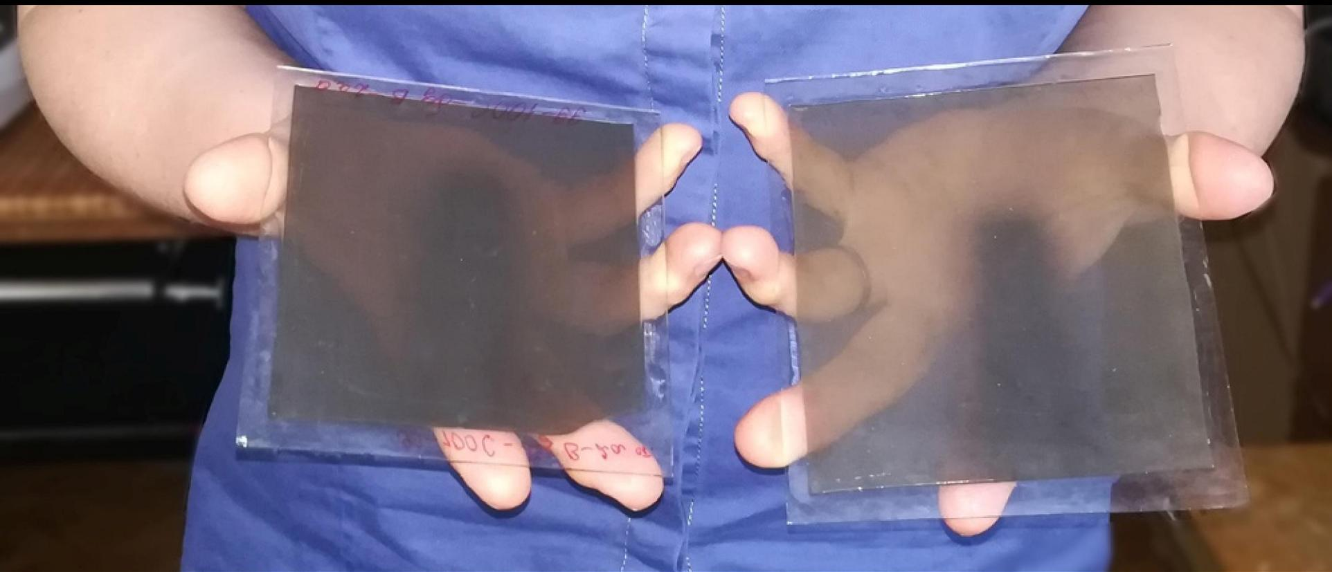
NTE samples enriched in boron (boric acid and borax) were irradiated for 30 min at the thermal neutron channel of the IBR-2 reactor JINR .
