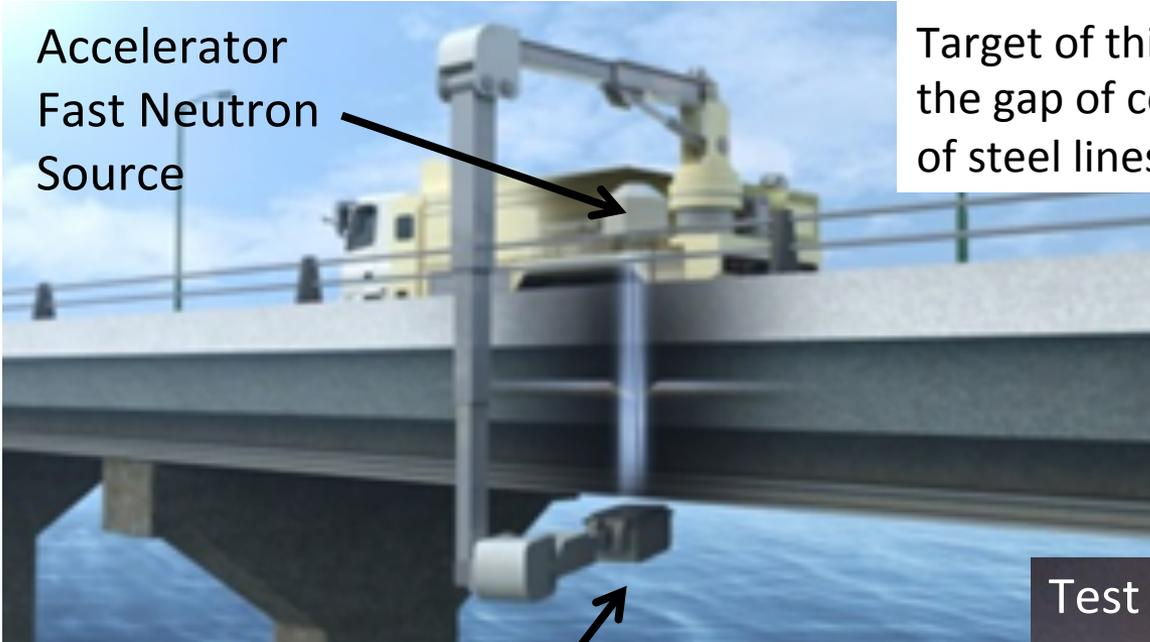
Target of this measurement is the detection of the gap of concrete and breaking or thickness of steel lines.
