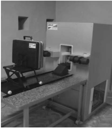
Fig. 1. Setup for the identification of hidden substances using tagged neutrons.
