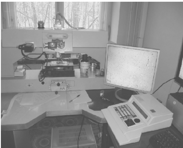
Fig. 8. PAVICOM-2 automated complex (Lebedev Physical Institute) created based on the MPE-11 microscope with controllable table, video camera, and image capture board; an image of a fragment of irradiated emulsion film is shown on the screen.
