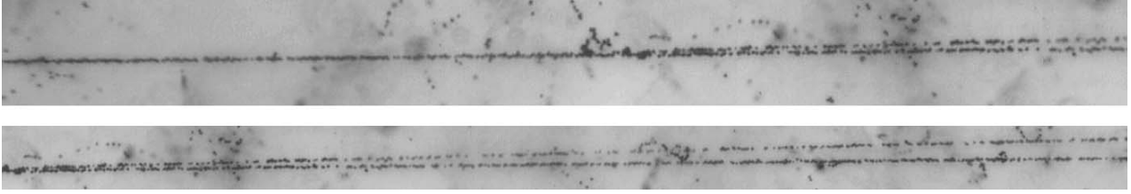
Fig. 4. Microphotograph of the charge-exchange fragmentation process ^{11}\text{B} \rightarrow ^4\text{He} + ^7\text{Be} . In the upper picture, one can see the interaction vertex and formation of two relativistic fragments within a narrow angular cone. With a shift along the fragment-emission direction (lower picture), one can distinguish a He fragment (upper track) and a Be fragment.
