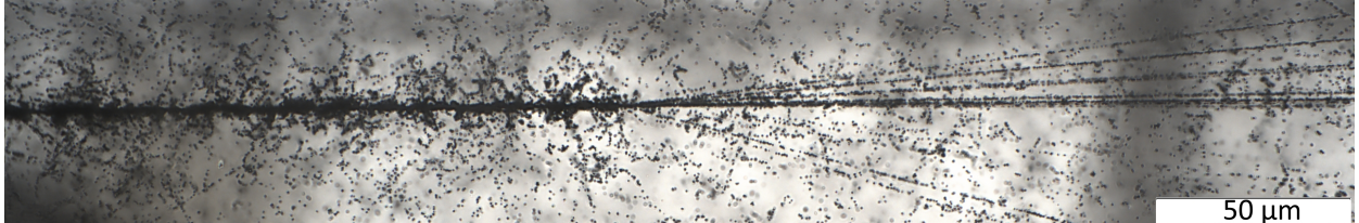
FIG. 1. Macrophoto of the peripheral interaction of the {}^{84}\text{Kr} nucleus with the energy of 950 MeV per nucleon having multiple formation of secondary He and H fragments.
