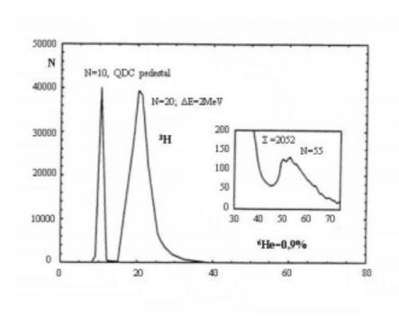
Fig.1 Signal spectrum of one of monitoring scintillation counters for magnetic transport channel tune corresponding to Z/A=1/3
