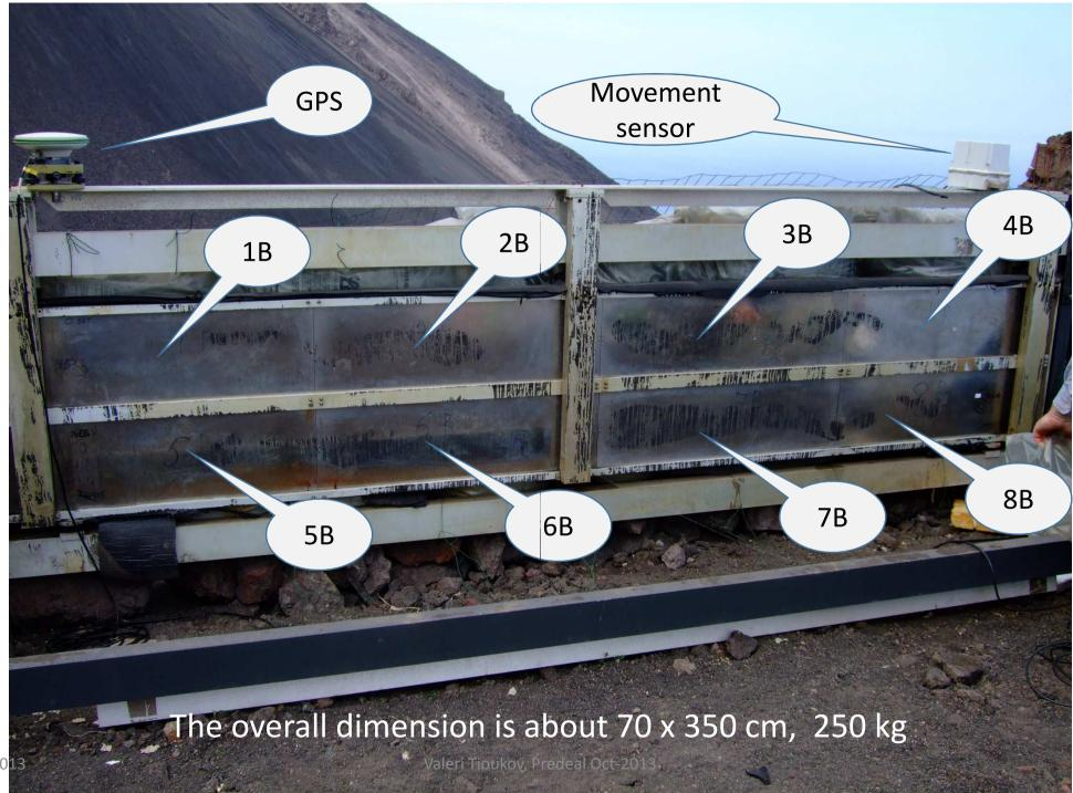
After 5 months of data taking we found the detector in a good shape well protected from sun heating and from moisture by rubber foam (armaflex) and by expanded clay
