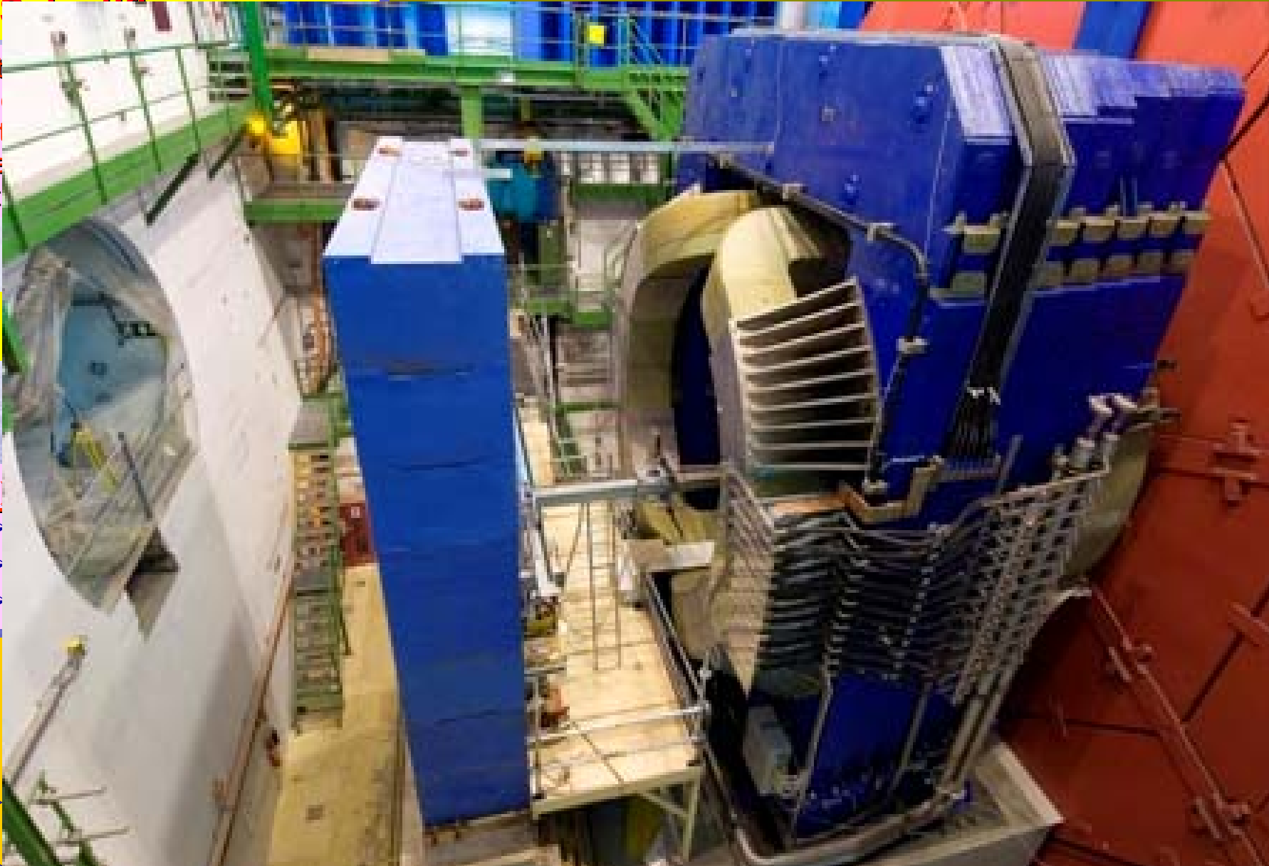
Very Large Dipole Magnet for Muon Spectrometer (9 x 7 x 3.5 m; 800 ton)
